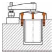
with 4 cap screws from above
